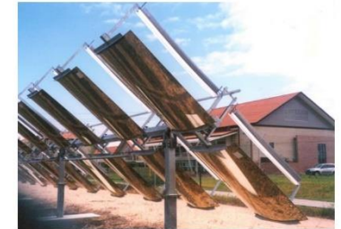
TAFE/Murdoch Rockingham – 250kW Mirror-concentrated PV system - Campus Energy Demand 50% Carbon-free
